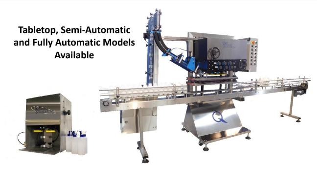
Spindle Cappers use two or more set of spinning disks to consistently and continuously thread caps onto containers as they move through the capping machine. Gripper belts and a stabilizer bar help hold the container and cap in place during the capping process. Spindle capping machines can handle a variety of continuous thread closures, including flat caps, flip-tops, sports caps, pumps trigger sprayers, CRC's and more!
